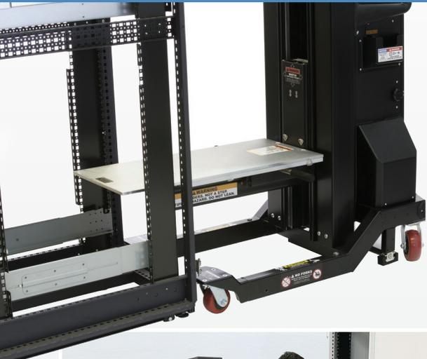
The ServerLIFT SL-500FX™ data center lift loads servers from the front with an extended shelf for deeper support into cabinets. This is especially useful when supporting servers for fixed rail and face-mounted installs. System integrators, test labs, or any facility with 5 ft (1.5 m) or more of space in front of the rack will benefit from its versatile, stable, and forward-sliding platform.
